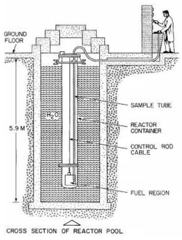
A diagram of the SLOWPOKE-2 reactor pool that is proposed to be filled with concrete. (Canadian Nuclear Safety Commission)
